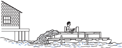
Blockage of boat exhaust by obstruction
