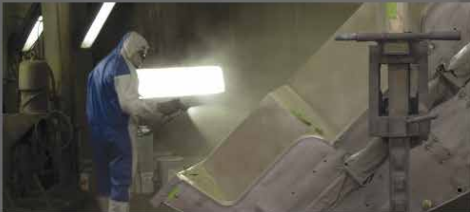
9 FULL PAINTED HULLS are first primed before painted and twice baked to provide showroom looks for years to come.
