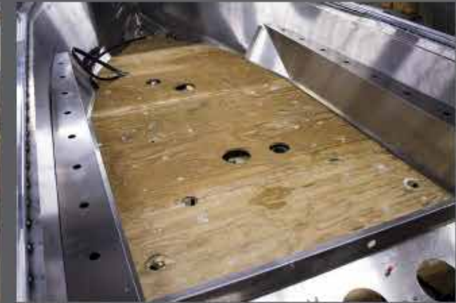
8 7-LAYER PLYWOOD FLOORS injected with urethane foam deliver maximum buoyancy, and all carpet and vinyl is installed with spray adhesive to avoid any loose fitting materials.
