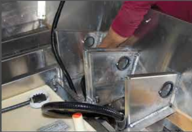
6 HEAVY GAUGE TRANSOM BRACES are through-bolted through the transom to allow for the high horsepower engines.
