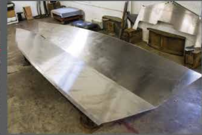
3 ONE-PIECE ALUMINUM BOTTOM is folded and molded to the greatest intrinsic shape.
