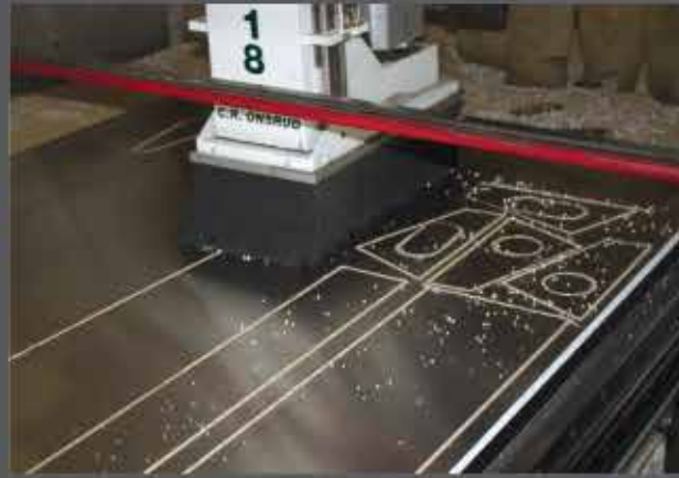
2 CNC ROUTED parts are cut out on a CNC router to the exact dimensions to fit perfectly into every boat.
