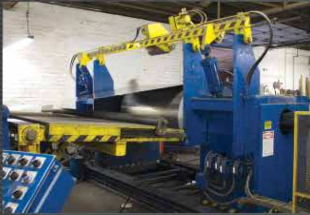
1 HEAVY GAUGE ALUMINUM is de-coiled into flat sheets that are ready to be cut, bent and molded for production.
