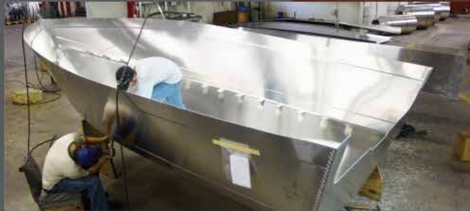
5 5052 H34 Marine grade 100 gauge aluminum resists dents, dings and corrosion for years of reliability.
