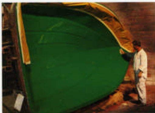
The 20-24 mm layer of high quality I.S.O. ortho N.P.G. Gel Coat is used to prevent cracking, crazing and provide UV stability to prevent fading.
