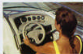
The console features a Quicksilver® Classic 3000 control box, Quicksilver instrumentation and an AM/FM cassette stereo.
