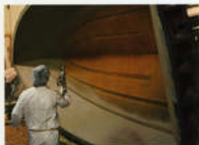
Spray Core ® 2000 on the sidewalls improves tensile strength over balsa or coremat. It also allows more strength and rigidity with less weight and gives more flex without cracking gel coat.
