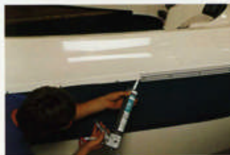
The hull and deck seams are sealed, thru-bolted and screwed. Then, a PVC gunwale molding is applied and screwed every 3" for a solid, secure fit which improves deck to hull integrity.
