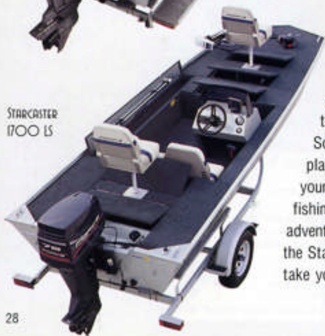
The high performance, reverse chine hull takes you to your fishing spot fast.
