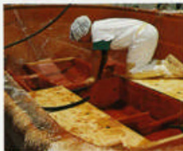
The floor system, made of 1/2" marine grade plywood, is encapsulated in fiberglass resin, screwed and laminated, preventing water intrusion.
