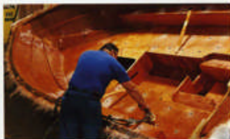
The integrated stringer system provides consistent strength. Stringers are laminated to the hull to increase strength and eliminate water intrusion.
