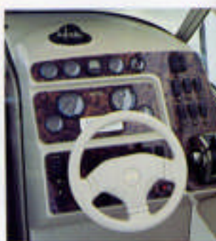
The command helm is home to a compass, tachometer, speedometer, voltmeter, oil temperature and fuel gauges, plus an hour meter, digital depth finder, and trim tabs.
