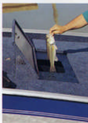
The Starcaster 1700 has both fore and aft 13 gallon aerated livewells.
